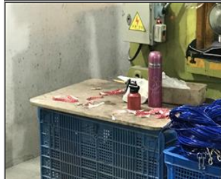
Photo of non-conformity 3 NC-chemical container without identification label.jpeg
